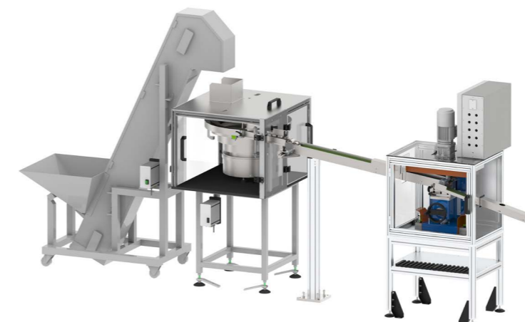
BM 73 EL with steep conveyor and separation with part recognition
